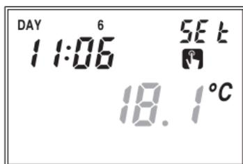
The display shows: DAY 6, 11:06, SET, a square icon with a circle inside, and 18.1°C (the 1 is flashing).
